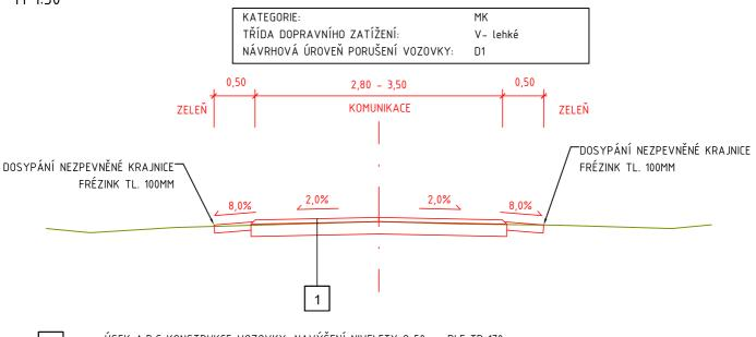
ÚSEK A.B.C KONSTRUKCE VOZOVKY, NAVÝŠENÍ NIVELETY O 50mm, DLE TP 170 1 ASFALTOVÝ BETON PRO OBRUSNÉ VRSTVY ACO 11+ 50 mm ČSN EN 13108-1:2008 INFILTRAČNÍ POSTŘIK Z KATION. ASF. EMULZE PI-E 0,80 kg/m2 VYROVNÁVACÍ VRSTVA ŠTĚRKODRŤ FRAKCE 0/32 ŠDΔ 0-100 mm ČSN 73 6126 ROZRYTÍ, UROVNÁNÍ DO SKLONU A PŘEHUTNĚNÍ PENETRAČNÍHO MAKADAMU 150mm CELKEM MIN. 300mm
